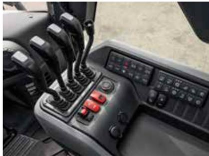
All control switches are conveniently arranged in a single location to enhance the operator's machine control.
