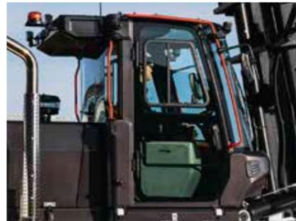
Upgrade operator comfort with the pressurized cab's two large air filters that effectively keep dust out. Plus, enjoy minimal noise at the driver's ear and reduced vibrations.
