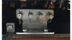
The pump, brake, and steering pressure measurement ports are independently built-in and centralized for easier pressure checking.
