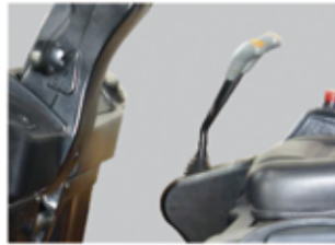
Hydraulic operating handle on the right side.
