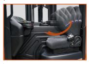
Shock-absorbing seat, adjustable backrest, and seat belt as standard.
