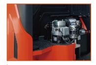
Low-noise gear hydraulic pump reduces the lifting noise of the whole vehicle.
