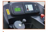
Multi-function color LCD instrument can display information such as steering wheel position, battery power, power alarm, fault code, running time, driving speed etc. The driving speeds of low, medium and high third gear can be set through the meter.
