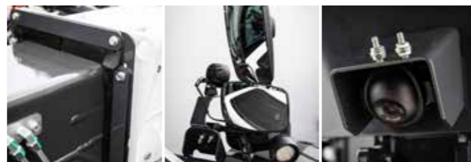
Dust protection on boom | Electric mirror with de-icing on right-hand side | Rear video camera
