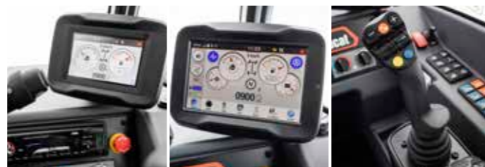
Standard 5" display with Bluetooth radio, microphone & loudspeakers | 7" touch display (Bluetooth radio with microphone & Job manager) | Smart joystick
